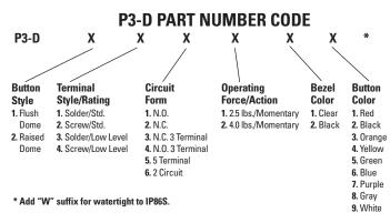
Example of building an OTTO Part Number: P3-D113124 is a switch with flush dome button, solder terminals, standard rating; N.C. 3 terminal circuit; 2.5 lbs. operating force, momentary action; black bezel; yellow color button.
